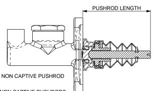
NON CAPTIVE PUSHRODS: CP5623 MASTER CYLINDER IS AVAILABLE WITH NON CAPTIVE PUSHRODS. THIS ENABLES THE REMOVAL OF THE MASTER CYLINDER WITHOUT NEED TO REMOVE THE PUSHROD FROM THE BRAKE PEDAL OR BALANCE BAR ASSEMBLY. PUSH RODS ARE AVAILABLE IN LENGTHS EQUIVALENT TO THOSE SHOWN ABOVE. PUSHROD TYPES: NCT - NON CAPTIVE PUSHROD THREADED 5/16" UNF
