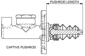
PUSHRODS ARE AVAILABLE IN THE FOLLOWING LENGTHS: 115mm (4.53") AND 160mm (6.3"). NON-STANDARD LENGTHS AVAILABLE ON REQUEST.
